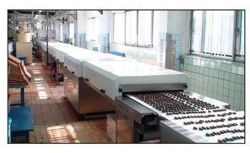
Module IntelleCool is combined cooling - dry tunnel for continuous cooling, drying, structurization of wide nomenclatures of confectionery, cottage cheese and other food masses. Module IntelleCool/Dry is supplied by system of automatic centering, cleaning and a belt tension, program-controlled system of speed control, separate adjustments of temperatures and modes at every stages if processing of a product. The cooled masses do not sticks to the cutting knifes (guillotine cutting).
